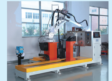
Robot seal welding
