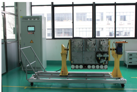
Fully automatic mechanical operation test equipment
